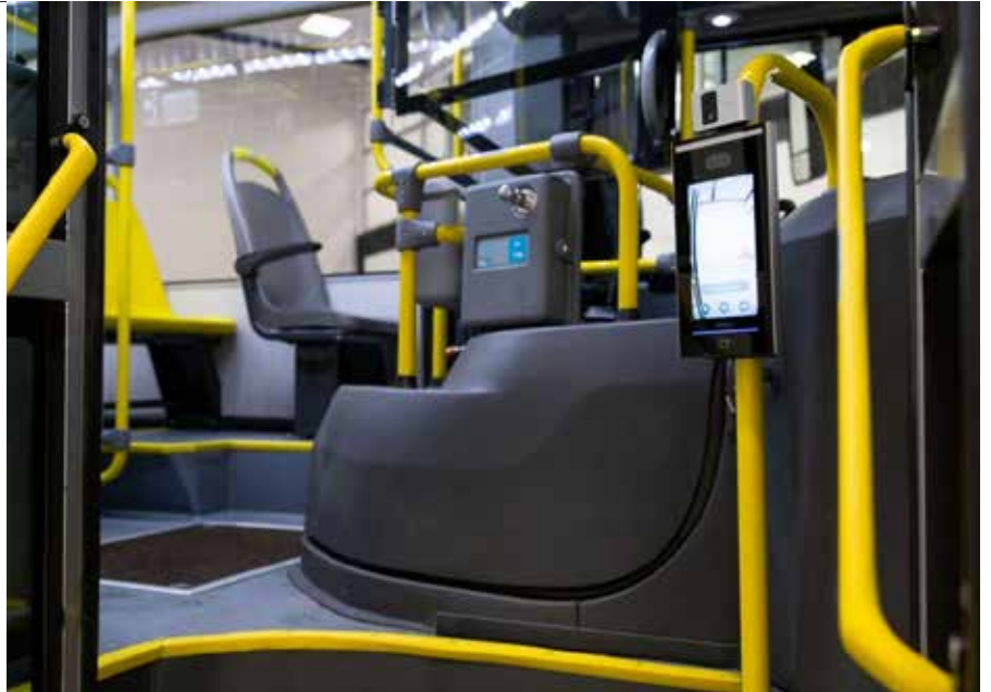
Entrance checking via facial recognition equipment in the buses
